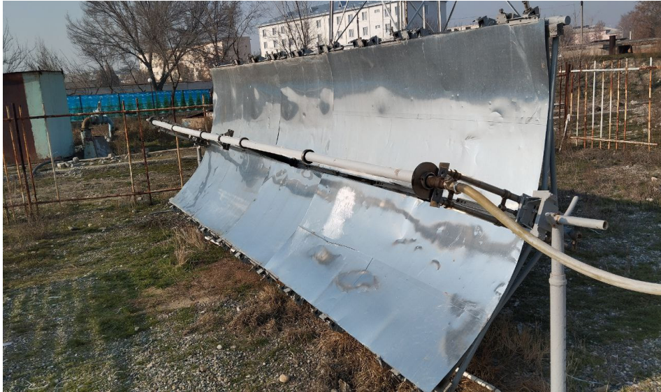
Fig.1. General view of the experimental PTC.
